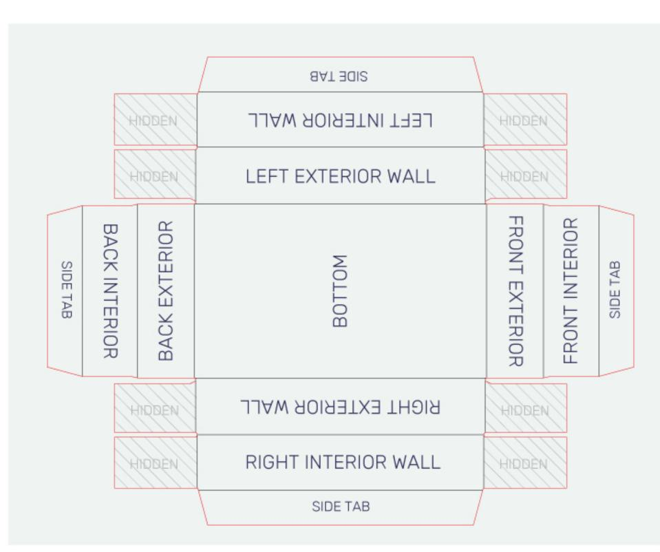
Note: After assembly, side tabs will rest on the bottom of the interior of the tray and will thus cover parts of the bottom interior design.
